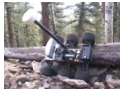
jBot uses ballistic behaviors to escape from entrapment.
