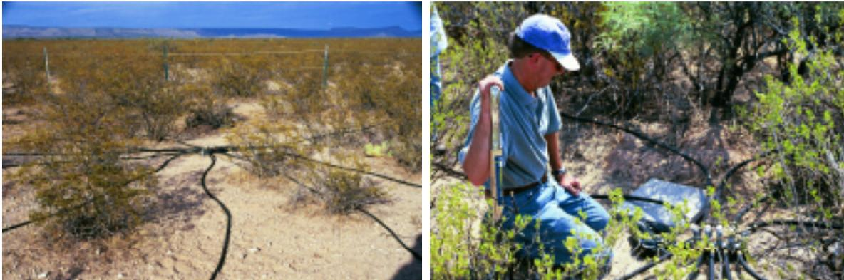
*Figure 8: The infrasound gage is connected to ten, 25-foot porous hoses for purposes of wind noise reduction. The radial distribution of the hoses at one of the array sites is pictured to the left. The manifold, which connects the hoses to the acoustic gage (buried and covered by a concrete plate), is shown to the right.*
