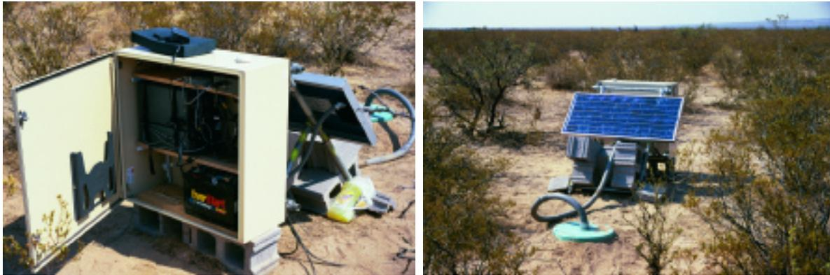
Figure 6: The equipment enclosure that houses the digitizer (Ref-Tek 72A-06), disk and battery is shown to the left. The solar panel is mounted on the opposite side of the enclosure and the seismic vault (blue) is located about 2 m from the enclosure (right)
