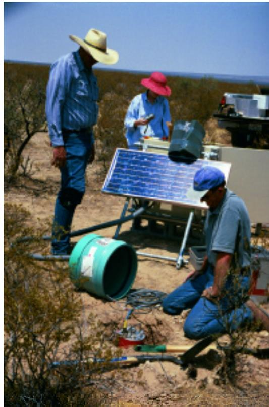
Figure 7: Installation of the vertical, GS-13 seismometer at the central array element, FTHAN0. The seismometer is being leveled on a cement slab at the bottom of the hole prior to installation of the blue protective cap.
