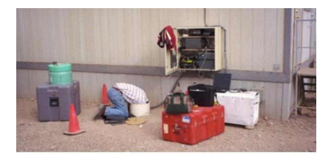
• Figure 6. Installation and leveling of the STS-2 seismometer in the Morenci vault.
