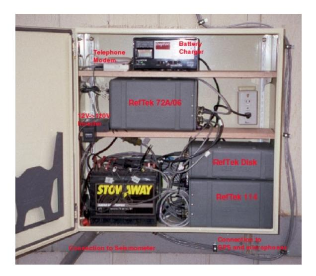
• Figure 3. Installed equipment at Morenci.
