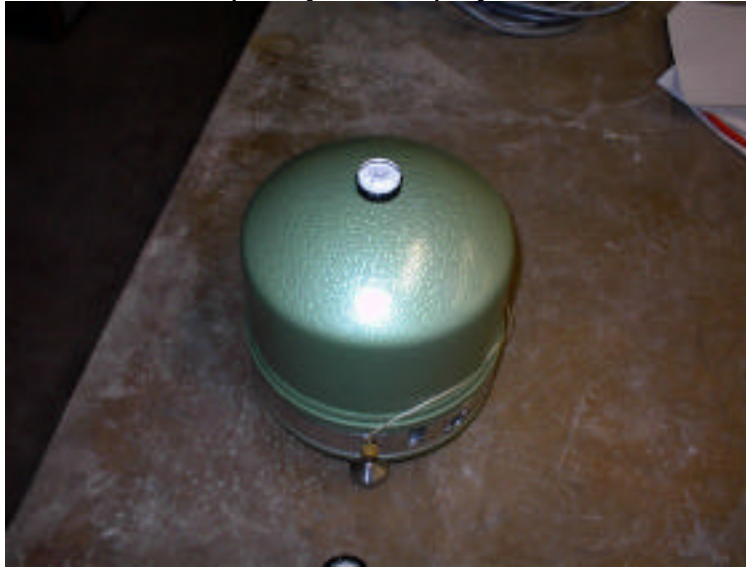
Figure 2. Strickheisen STS-2 three-component broadband seismometer.
