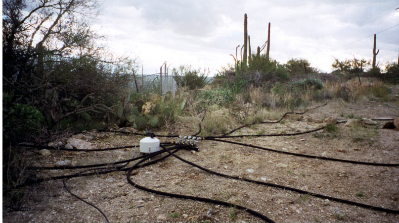
Figure 6a: Infrasound site TUC0, which is directly above the seismic vault. The Chaparral Model 2 acoustic gage is the small white instrument to the left. The summing manifold is connected to ten, 25 foot porous hoses.
