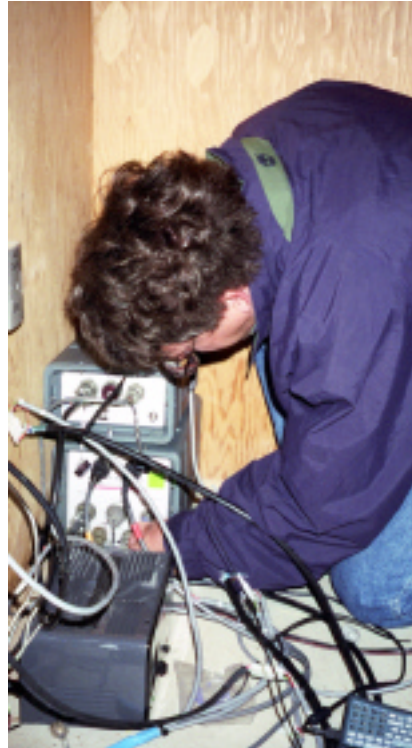
Figure 4: Installation of the Ref Tek 72A-06 digitizer, disk and battery charger in the seismic vault at TUC.
