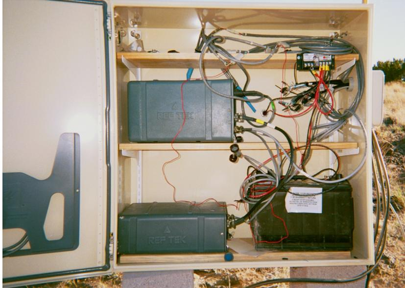
Figure 7. Installation of the RefTek 72A-06 digitizer, disk, and battery charger in the solar powered enclosure at Wupatki.
