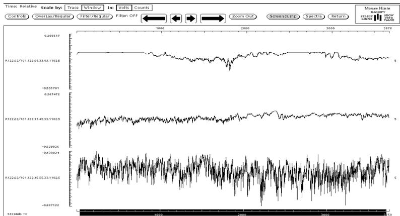
Figure 17. Wind speed recordings for three different hours. Anemometer output is sampled once per second. The top trace includes several minutes of dead calm. The bottom trace was recorded during high winds. Increasing wind velocity results in a negative (downward) deflection of the trace.
