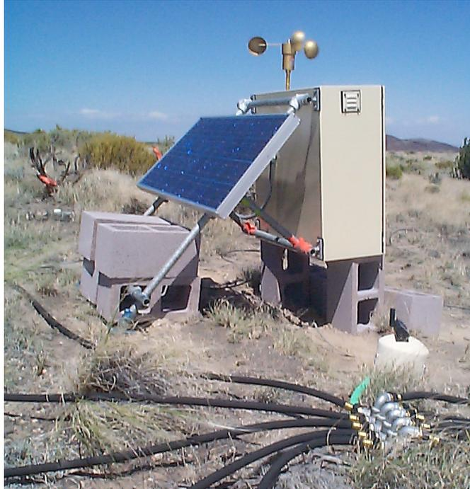
Figure 8. The solar powered enclosure for Wupatki where the digitizer (RefTek 72A-06), disk and battery are located. The solar panel is rated at 12 volts/ 64 watts and faces approximately south. The acoustic sensor and manifold are shown in the foreground.
