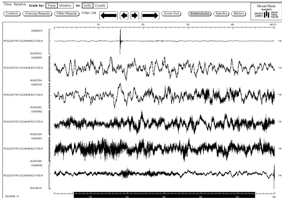
Figure 19. Site WUAZ0 recorded at 250 samples/second during 6 one-minute sampling periods. The high frequency noise on traces 4 and 5 is probably aircraft or vehicle noise. The spike on trace 1 is probably the result of a footstep or a vehicle door slam.
