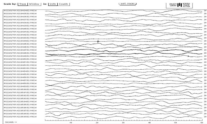
Figure 18. Overview of the channel recorded for ambient background monitoring. Each trace is only 60 second long and was recorded at 250 samples/second. The small signal on the 11th trace is probably a result of a footstep near the
