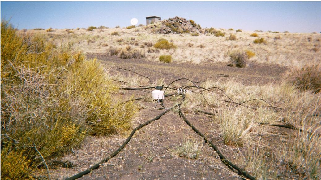
*Figure 13. Site WUAZ3 looking northwest towards WUAZ. The stiff connection cable has not yet relaxed enough to lie flat upon the ground. Even in the air, it is unlikely to result in significant additional wind noise.*
