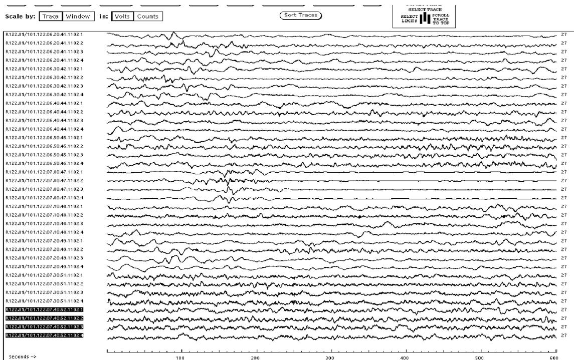
Figure 14. Ninety minutes of data from Julian Day 122 recorded at Wupatki. Nine continuous, 600-second data segments are plotted. Each set of four traces represents the data from the four acoustic sensors WUAZ1, WUAZ2, WUAZ3, WUAZ0. In this display the traces are trace independently scaled. Actual data traces for channels 3 (WUAZ3) and 4 (WUAZ0) are about  $\frac{1}{4}$  that of the other two channels.
