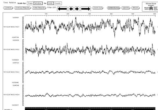
Figure 15. Ten minutes of data from infrasound sensors WUAZ1, WUAZ2, WUAZ3, and WUAZ0. The last two sensors have about 1/4 the gain of the first two.
