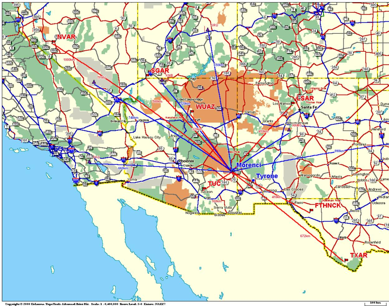
Figure 1. Map illustrating the existing and proposed stations that will make up the Western US seismo-acoustic network. Seismo-acoustic stations are shown as red flags, seismic only as purple triangles, and sources as blue pins.
