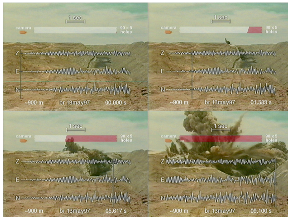
Figure 17a: Video, ground motion and simple model for a second cast shot in a different mine. This cast shot utilizes a simple shooting pattern where echelon boreholes in each row are detonated every 100 ms. This pattern produces the regular nature of the resulting seismograms.
