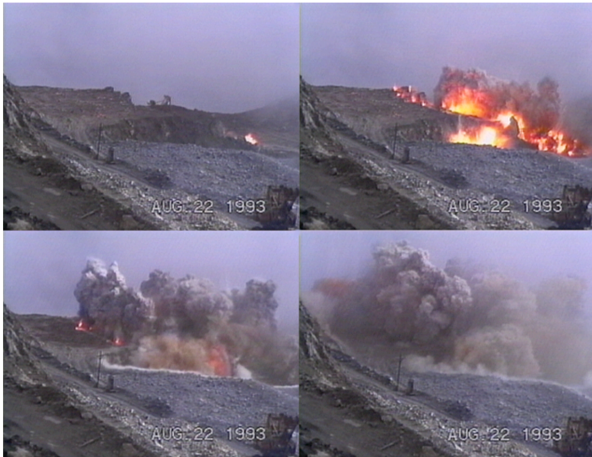
Figure 14a: Video images from a hard rock fragmentation shot. In this shot each row is detonated simultaneously with a 100 ms delay between rows. Note the lack of stemming and the surface explosions that are captured in the video.
