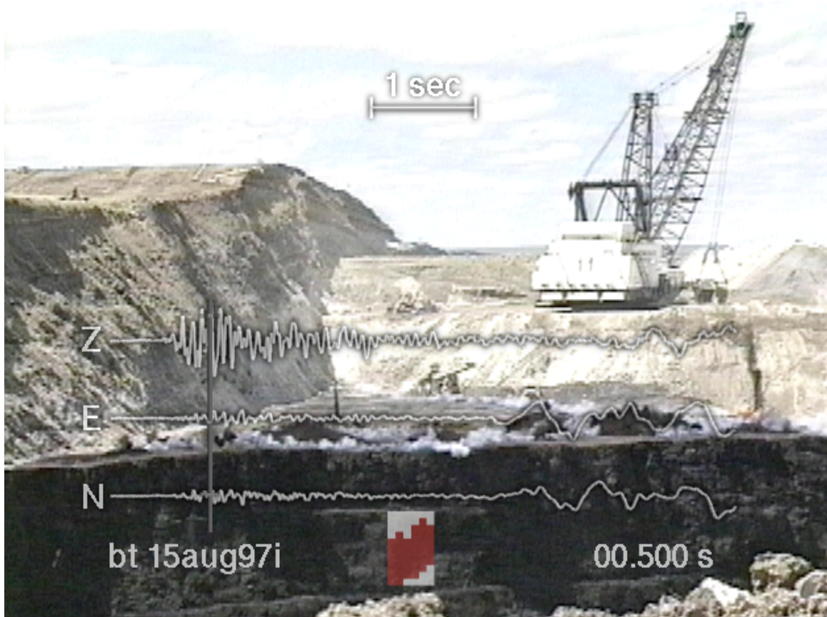
Figure 8: Same as Figure 7 with a simple two-dimensional model of the blast time correlated with video and ground motions. Pixels in the model represent individual blast holes and turn from white to red at design detonation time.
