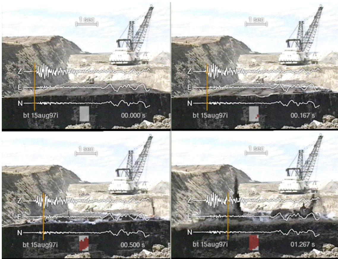
Figure 13a: Video images combined with ground motion and two-dimensional model for a small coal fragmentation shot. These are the images used to demonstrate data processing and model combination in Figures 5-10. The short duration of this type of explosion is quite apparent in the seismic waves.
