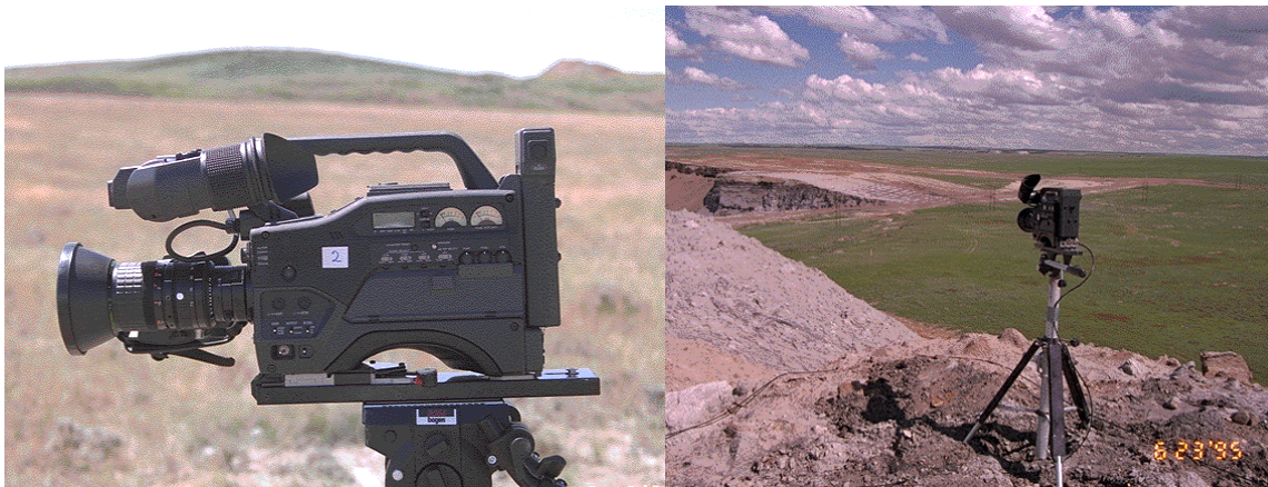
Figure 1. Installation of a Sony EVW-300 Hi-8 video camera overlooking a cast shot. The coax cable is connected to a companion camera so that they are Genlocked (frame-by-frame sync between two cameras).
