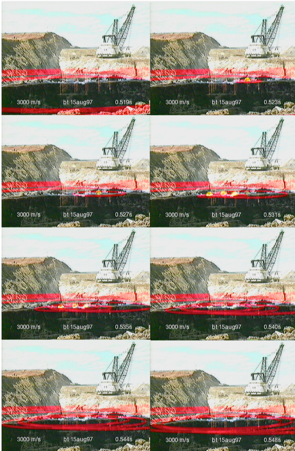
Figure 16: Eight video images with superimposed 3D model from the coal shot. The model is sampled at 240 images/s and superimposed on de-interlaced video data. The eight images represent 1 video frame or two de-interlaced fields emphasizing the temporal resolution of the video data relative to blast phenomena.
