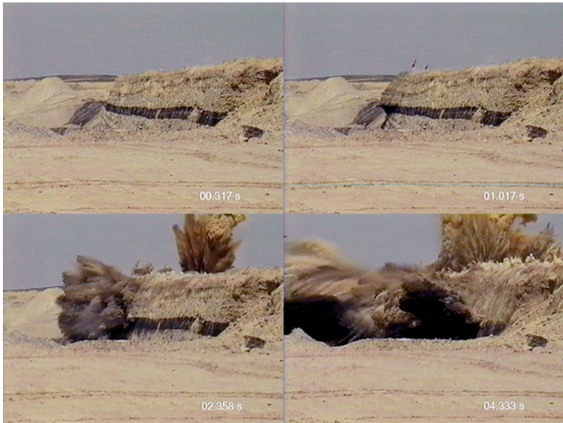
Figure 19: Four video images from a shallow overburden cast blast. Evidence for damage to the coal during the blast is seen in the image at 1.017 s and 4.333s.
