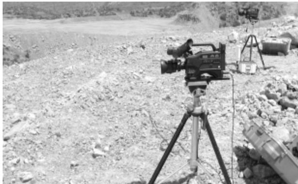
Figure 5. GPS locked stereo video camera recorders are setup at a convenient location with a good view of the shot. The cameras are synchronized to each other and to GPS time. These are standard video cameras and after post processing, one frame is produced each 16 ms from each camera. The use of two cameras gives additional redundancy and can provide stereo images of the shot.
