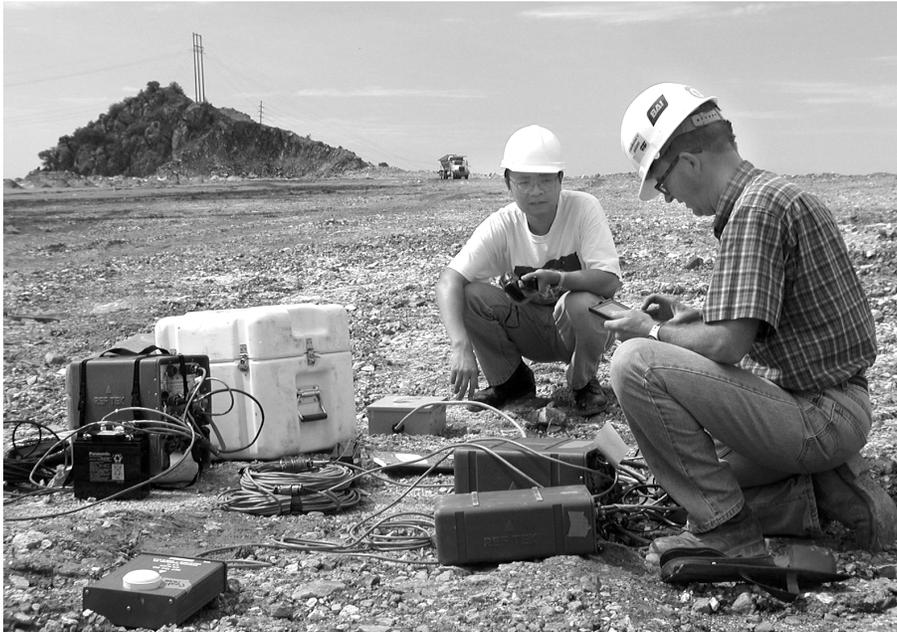
Figure 2. Two people install one of the four near shot monitoring stations. This station includes two three channel recording systems running at 1000 samples/second continuous recording output from a 3 component 1 g accelerometer and a 25 g accelerometer. The pattern is just below the hill in the background.
