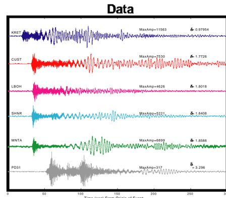
Figure 2. Observed vertical component seismograms of event (white triangle in upper panel of Figure 1) at all stations. (Seismometer for PD31 is KS54000. Other stations use STS-2)
