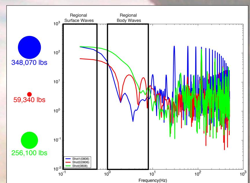
Near-source accelerograms provided in-mine documentation of blast timing. The spectra of the design shot times are compared with the displacement spectra determined from acceleration measurements. The similarity of the spectra up to 20 Hz suggests that source timing effects are responsible for a decrease in amplitude for the largest shot. Above 20 Hz, the spectra diverge since the impulse time series does not include the corner frequency of the individual blasts.
